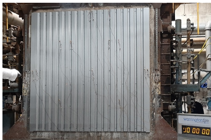
Image 1: Twin-Therm® Wall Test Set Up
